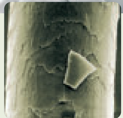
Size comparison: pearlescent pigment on a human hair under an electron microscope.
