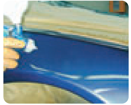
Apply clearcoat to the complete part. Make sure that the clearcoat application is thin in the area next to the adjacent part.
